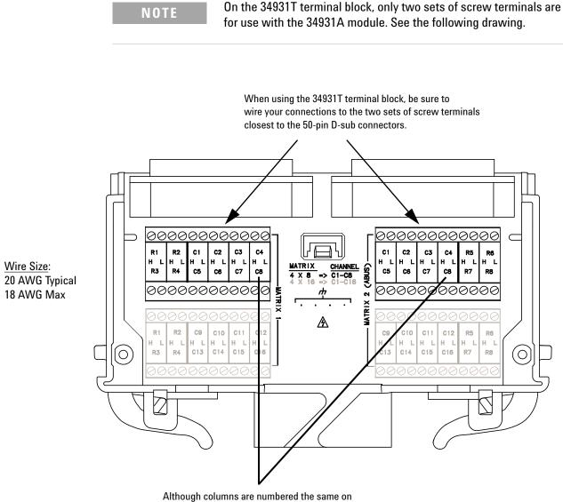
Although columns are numbered the same on Matrix 1 and Matrix 2, they are electrically separate from one another (e.g., Col C8).
