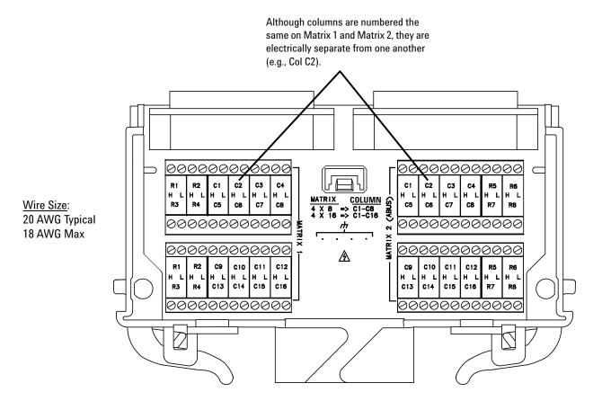
When using the 34933T terminal block for 2-wire mode, access is provided to the bypass columns through the columns labeled C9 through C16. Follow this wiring convention shown in the table below for both matrices.
